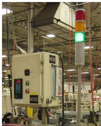
Figure 7. An example of an LED stack light, clearly communicating the status of a machine.
