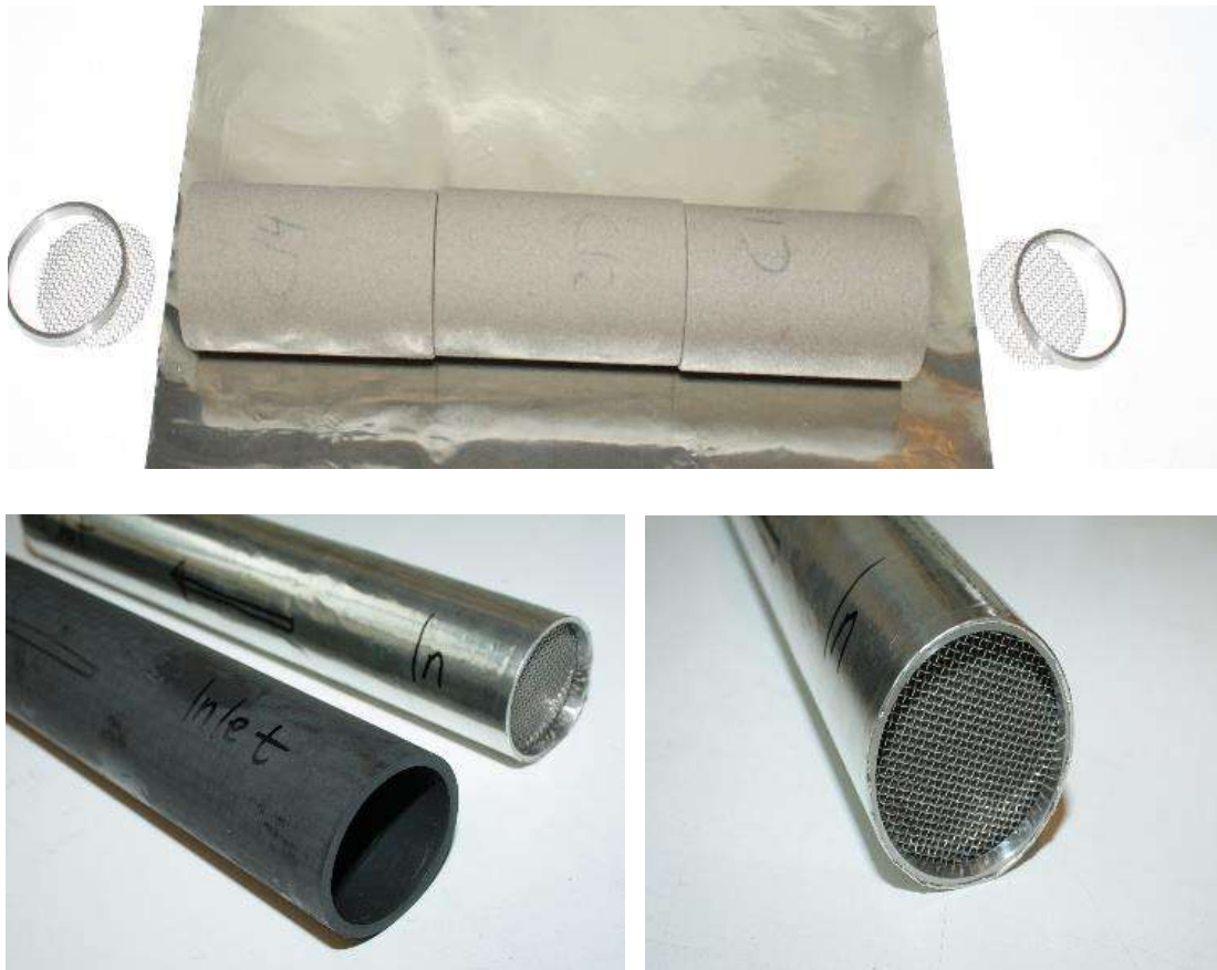
Figure 7. Three core plugs and the appliance for mounting the cores in the core holder.
