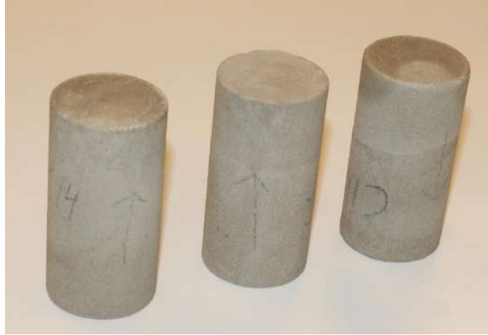
Figure 13. The core plugs after \text{CO}_2 flooding experiment. The inlet and outlet appear to be wet (higher content of water) and the core plug in the middle seems to be dry.
