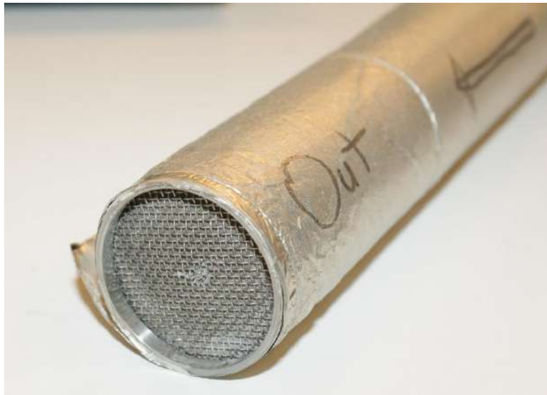
Figure 14. the core samples outlet after opening the core holder after CO_2 flooding. The salt in the middle of the filter is shown in this picture. This outlet is the original outlet and further became inlet after changing the flow direction.
